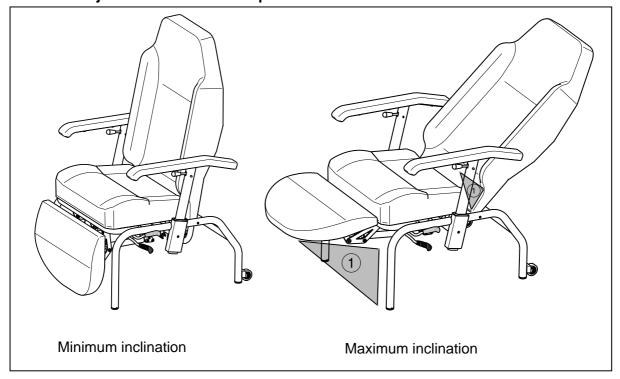
The angle of the backrest and the legrest can be adjusted by means of a pneumatic gas spring.
