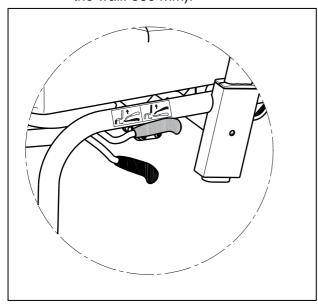
Lightly pull up the grey lever, the pneumatic spring is released and the backrest can be moved into the desired position. If you let the lever go again, the pneumatic spring is blocked and the backrest stops at the desired position (inclination: 10° - 45°).
