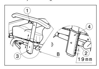
Pull the lever of the armrests ① upwards (in the direction of the armpad).
