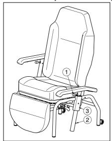
To lower the armrest for a sideways transfer, pull the lever ① and guide the armrest down to the lowest possible position.
