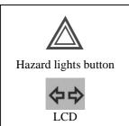
To put on the emergency lights, press the triangle button, at the same time the button will flash red and the indicator lights buttons turn green.
