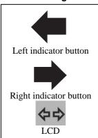
To put on the indicator lights, press the desired button (left = left indicator, right = right indicator). At the same time the button will turn green and has a sound from a horn. Press the Button again to turn the indicator off.
